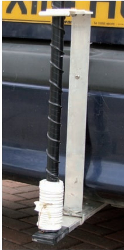
Fig. 5: The final tuning must be done while the antenna is mounted on the vehicle to be used. Chris G4DCH recommends using a suitable antenna analyser.
